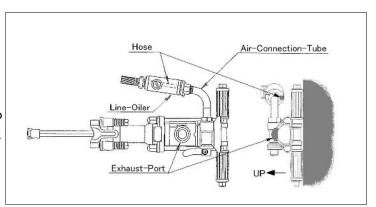
The case that the Hose in the Line-Oiler is set upper than the Exhaust-Port, Oil in the Line-Oiler will leak if the Air hand Hammer is left on the ground with the Exhaust-Port upward.
